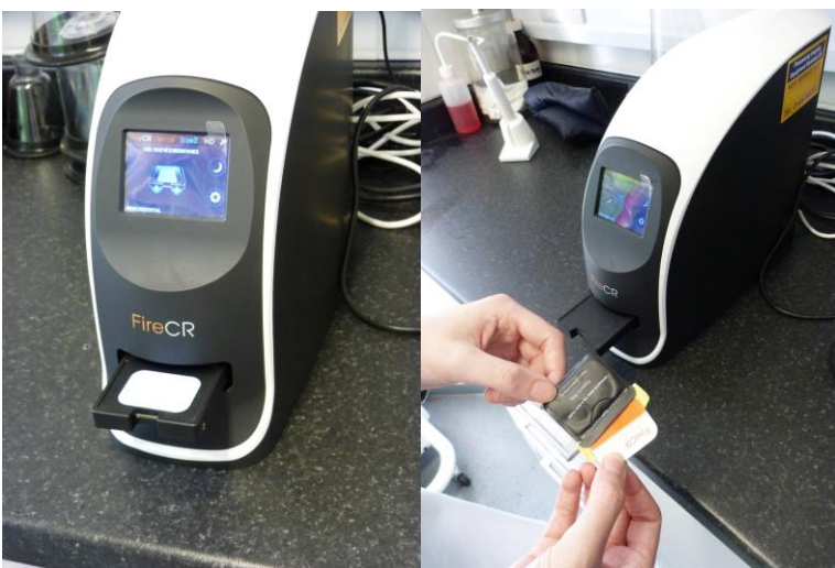
Processing Fig 16-17: Processed and cleared PSP delivered on tray for placement into protective envelope and re-use.
