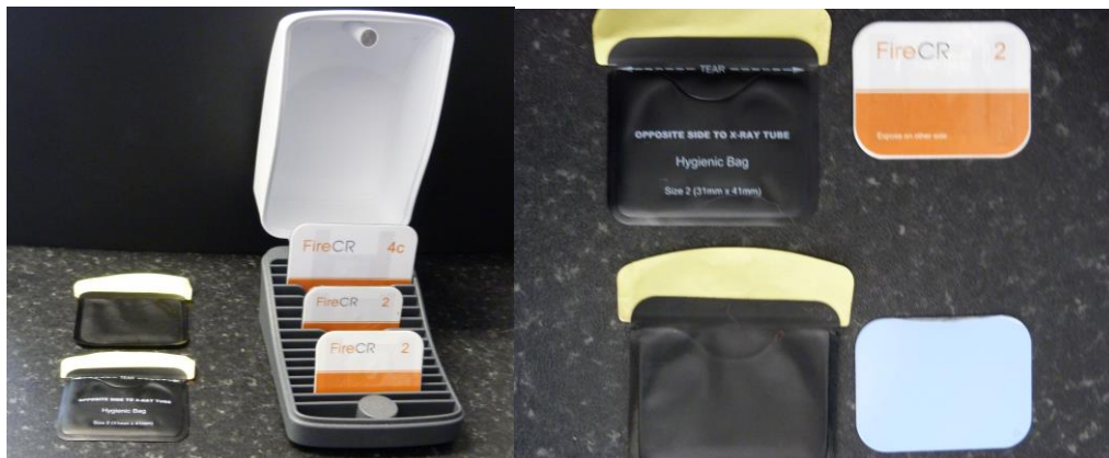
Processing Fig 7-8: PSPs and protective envelopes; plain sides of envelope and plate (blue, active coating) align.
