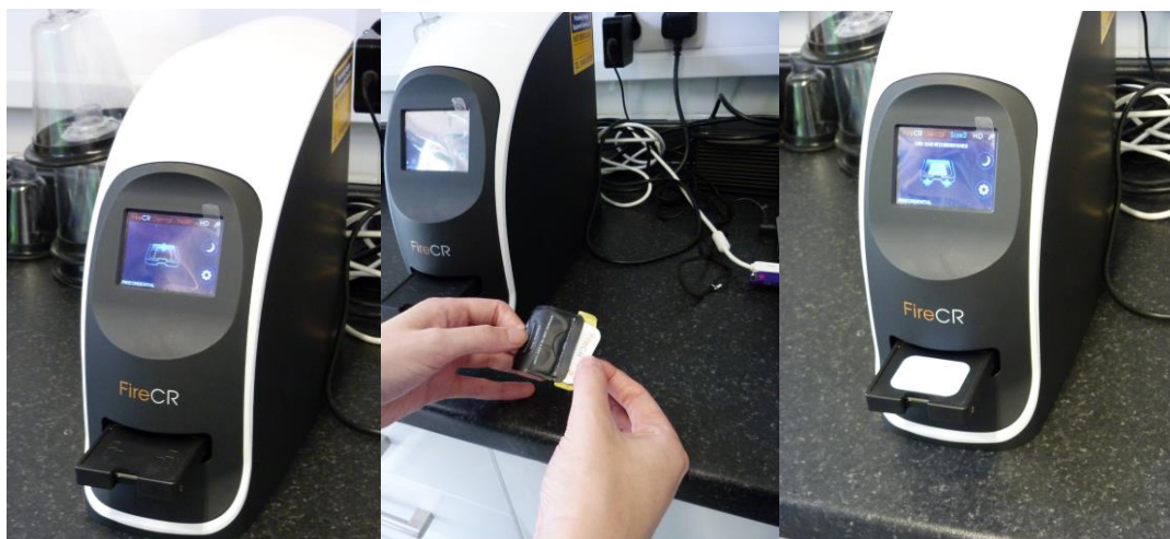
Processing Fig 10-12: Fire CR PSP reader – note magnetic area of feed-tray for easy alignment of PSP; size 2 plate removed from envelope and positioned.
