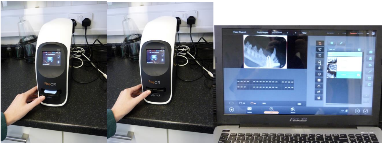
Processing Fig 13-15: Tray pushed inwards then automatically taken into reader; rapidly processed image appears on screen. Clear, simple software is advantageous and encourages use.
